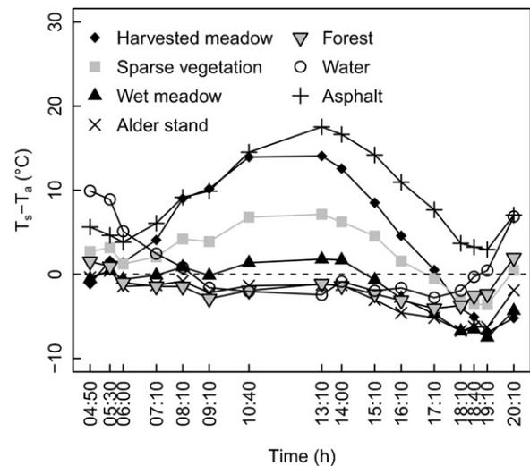
Fig. 5. Temperature differences  $T_s - T_a$  between surface  $T_s$  and air temperature  $T_a$  (at 2 m above ground) at all studied localities.
